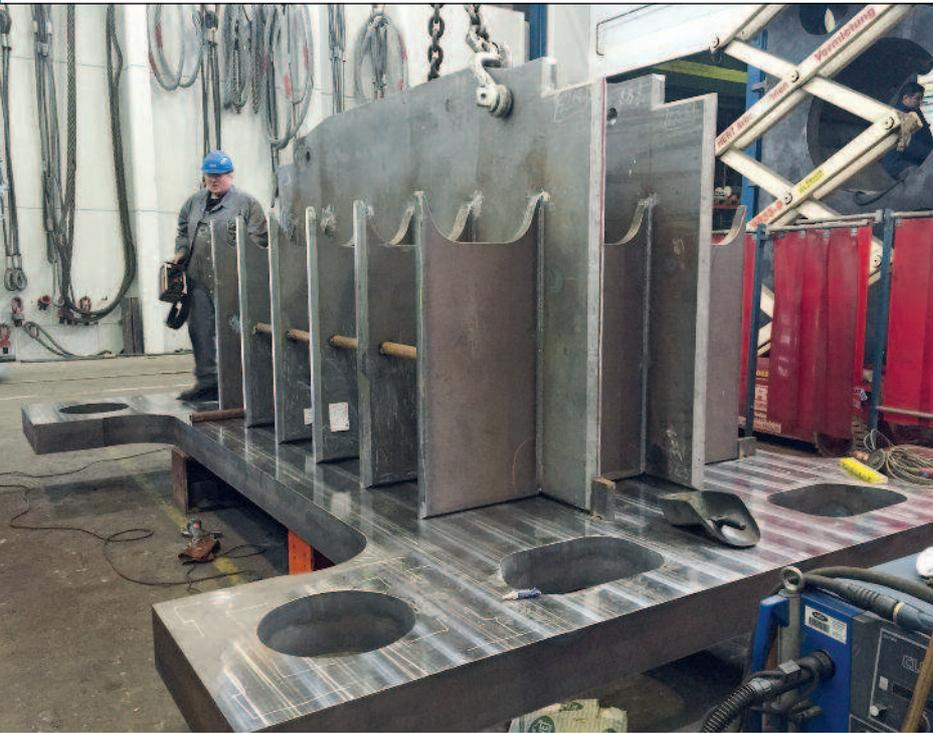
*The SAW narrow-gap welding method allows us to weld thick walls, up to 500 MM.*
